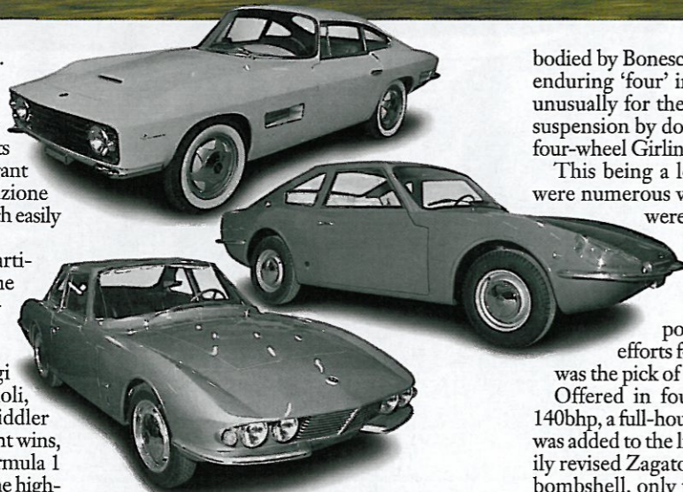
OSCA nominations, from top: '61 Boneschi; glassfibre-bodied Corbetta-styled '64 1050, based on Fiat 850; late-model MV used Ford Taunus 1.7-litre V4 engine
